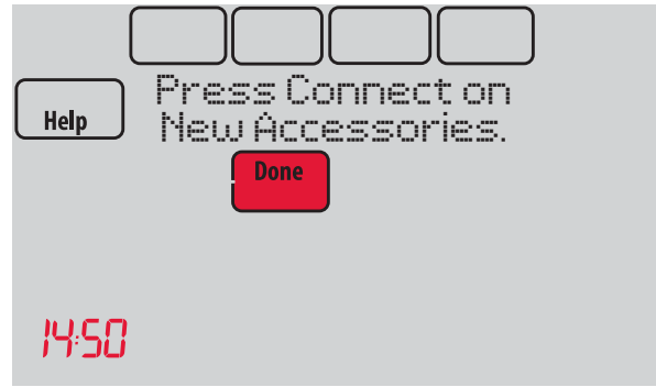
Fig. 35. Thermostat in listening mode.
