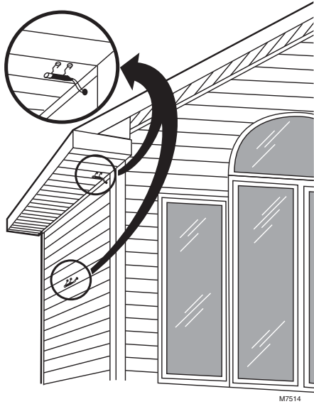
Fig. 73. Typical locations for C7089U1006 Outdoor Sensor.
